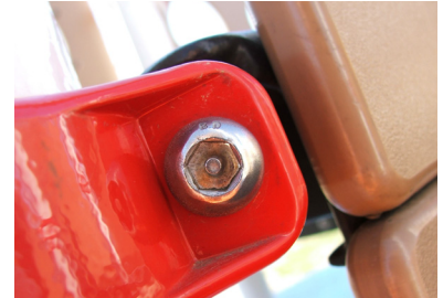
Loose bolt poses pinch hazard.
